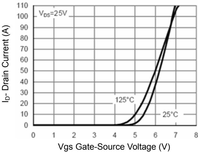
Figure 2 Transfer Characteristics
