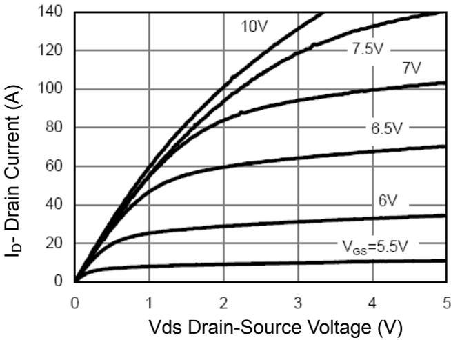
Figure 1 Output Characteristics
